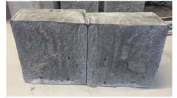
Investigation of depth of water penetration under 5 Bar water pressure for 72 hours. No water penetration was found.
