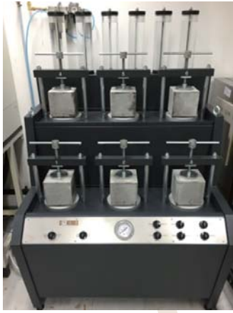
Water permeability apparatus
