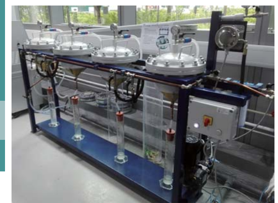
Automatic concrete water permeability apparatus (CRD-C 48-92)
