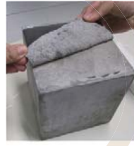
Investigation of depth of water penetration under 5 Bar water pressure for 72 hours. No water penetration was found.
